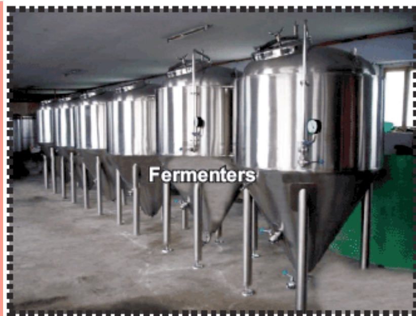
Figure 17.5: Fermenters used in food and pharmaceutical industry
