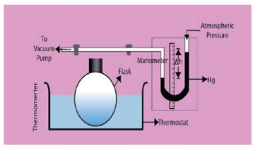
Fig. (4.11) Measurement of vapour pressure of a in the heights of the columns of-Hg in liquid by manometric method
