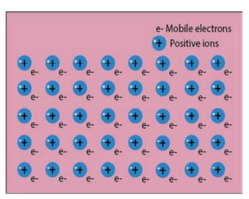
Fig (4.20) Positive ions surrounded by mobile electrons
