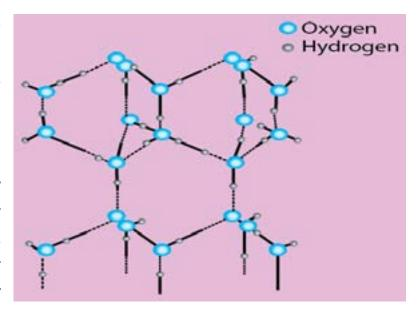
Fig (4.8 b) Structure of ice
