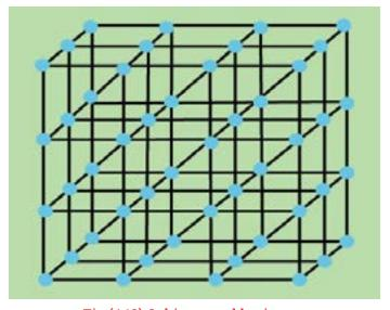
Fig (4.13) Cubic crystal lattice
