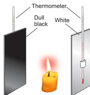
Figure 9.16: A comparison of absorption of radiation.
