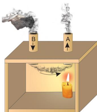
**Figure 9.8:** Smoke showing the path of the convection.
