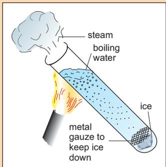
Water is a poor conductor. Water at the top in the test tube starts boiling after getting heat from the burner without melting ice.
